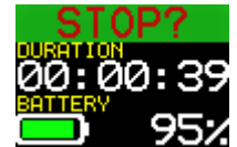
Color coded display showing remaining battery life
